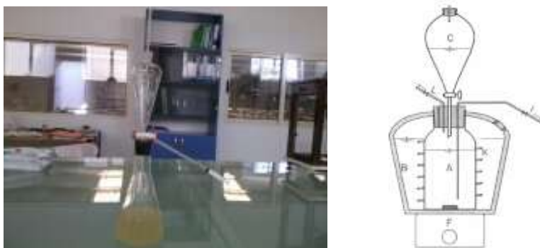
Figure 1. Apparatus built to study disinfection kinetics of \text{ClO}_2
